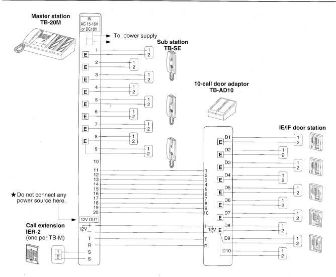
TB-AD10, 10-call door adaptor may be wired to any # terminal on TB-M or TB-G add-on selector, connecting max. 10 IE/IF door stations. Features two-way calling and communication with door station, including optional pretone. Set the switch to ON position, if pretone to door is required.
